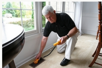
Stan Broyles, owner of Stan Broyles & Associates, uses a velocity meter to measure the air flow at a client's home in Rochester. Broyles specializes in balancing air flow to eliminate hot and cold rooms. (Kiya Gibbons / Special to The Detroit News)
